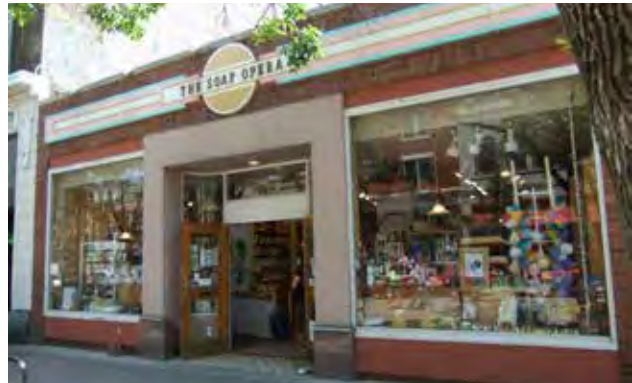
Fig B.4.D.2: High levels of transparency are required between the heights of 2 and 12 feet on street-facing facades.
