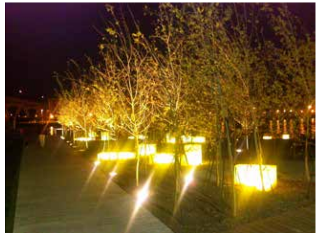
Fig. A.10.C.5: Light fixtures on the ground prevent landscaping elements from blocking light and creating dark spots.
