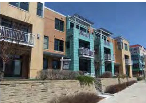
Fig B.3.D.6: An elevated landscaped area and a decorative wall create a division between public and private space.
