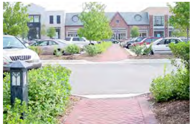
Fig. A.7.C.3: An attractive walkway through a parking area minimizes pedestrian conflicts and improves the appearance of the development.
