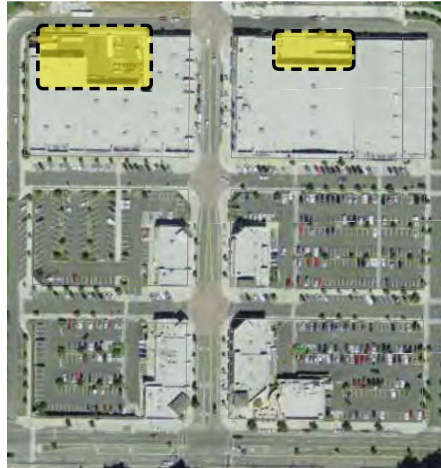
Fig. A.9.C.1: Service areas located away from public areas of the site.
