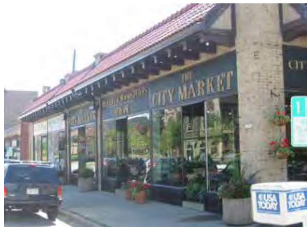
Fig B.4.D.2(2): High levels of transparency are required between the heights of 2 and 12 feet on street facing facades.
