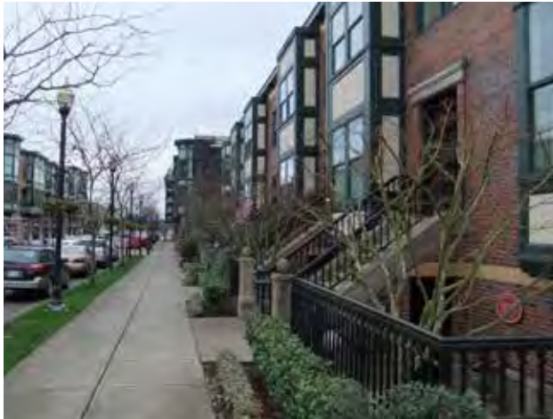
Fig. A.3.C.5: Townhomes utilize a small setback defined with landscaping and stoops to transition from public space.
