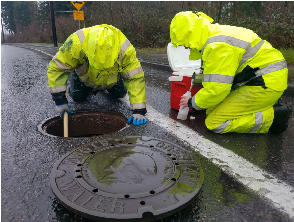
Gresham Stormwater staff taking samples of rain runoff from a manhole on the street.
