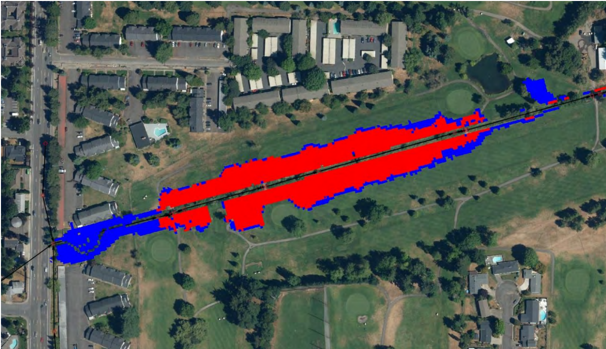
50-year existing-conditions flood extents (blue) overlaid with potential project flood extents (red).
