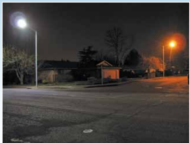
LED streetlight (left) versus traditional streetlight (right) shows brighter and whiter light. PNNL photo.
