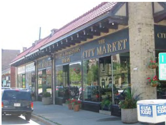
Fig B.5.S2.a: High levels of transparency are required between the heights of 2 and 12 feet on street facing facades.
