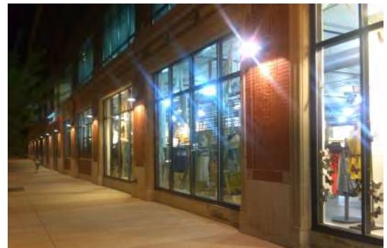
Fig. A.7.G1.b: Storefronts and wall sconces create appropriate illumination levels on a pedestrian walkway.
