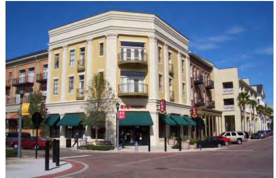
Fig B.6.S2: Facade sections fronting the Gateway intersections shall be at least 3 occupiable stories.
