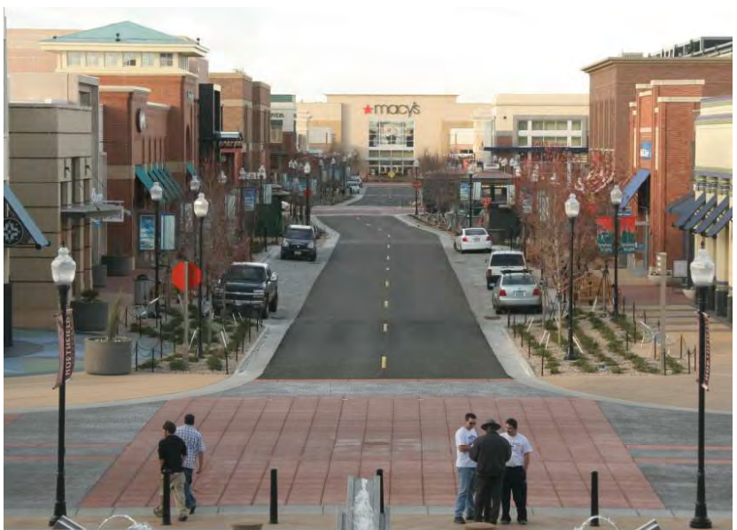
Fig. A.1.G4.c: Pedestrian conflicts are minimized by limiting driveways and providing visually distinct crosswalks.
