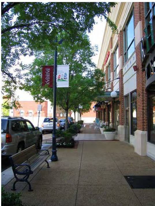
Fig. A.5.S6.c: A streetscape which features decorative paving, trees in planters, benches and pedestrian-level light fixtures compliments the abutting building with high levels of transparency and frequent entries.
