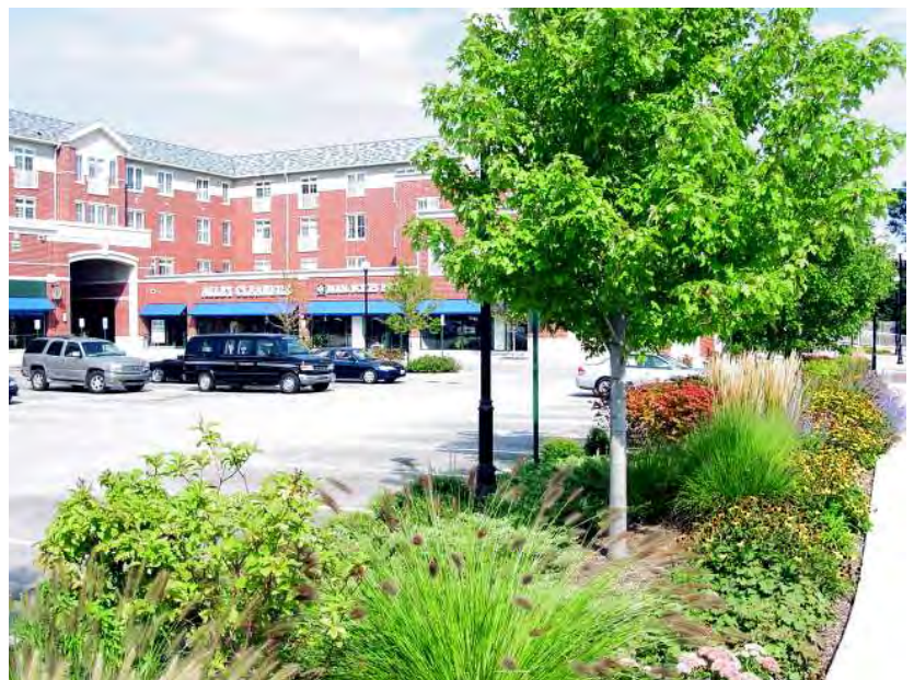
Fig. A.4.G2: A landscaped area is used to divide a large parking area into series of smaller lots.
