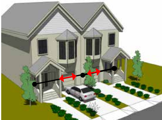
Fig. A.4.S11: Garage opening widths are less than 50 percent of the facade width of the unit they serve.
