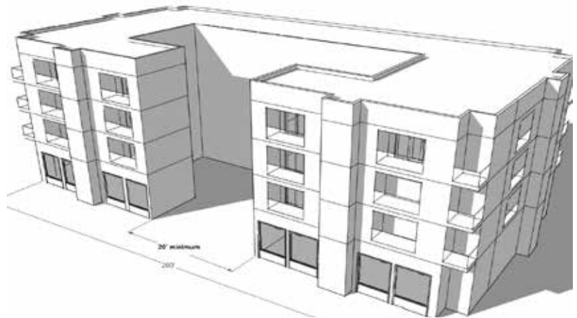
Fig. B.1.S4: Structures facing a street can increase horizontal length to 200 feet by providing an internal courtyard with a minimum 20 foot width.
