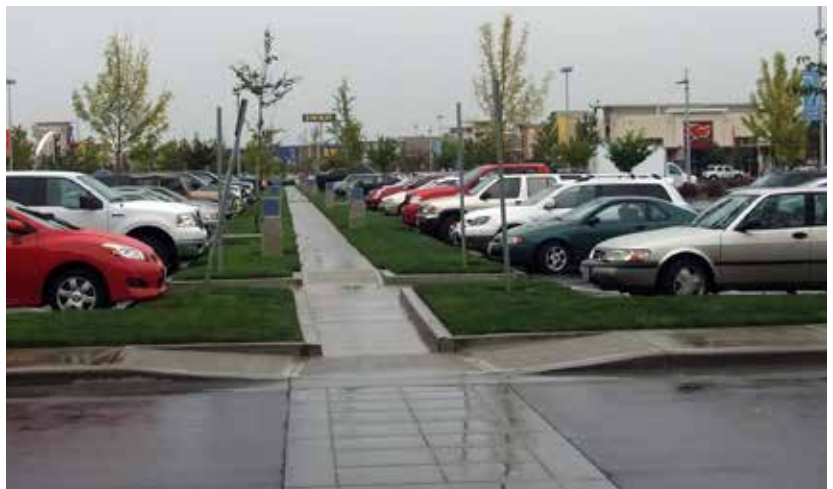
Fig. A.3.S2: A pedestrian circulation route which is separated from parking stalls and utilizes contrasting paving where crossing auto traffic routes.
