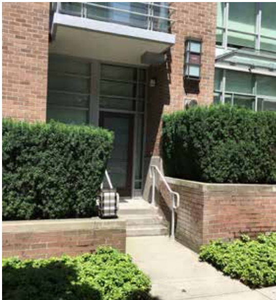
Fig. B.3.S8: A ground floor entry is separated from the public realm (the sidewalk) with an elevated entry and raised planters.
