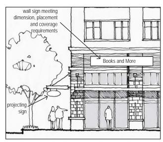
Fig. B.4.d.1 & 2: Ground-floor sign diagram
