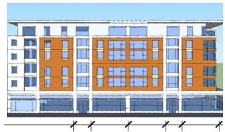
Fig. B.2.c.4: Belt line above the ground level and regular cadence of bays and storefronts.
