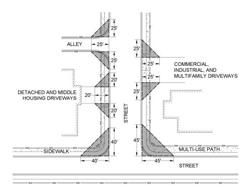
A Clear Vision Area for intersections of streets and an alley shall consist of a triangular area, one side of which is the back of the street curb and one side of which is the property line along the alley as extended to the street curb, for a distance specified in the table below, and the third side of which is a line joining the non-intersecting ends of the other two sides.
