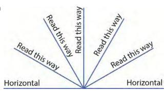
If possible, lettering and dimensions shall be placed so they may be read from left to right as viewed from the bottom of the sheet or from bottom to top when viewed from the right side of the sheet.
